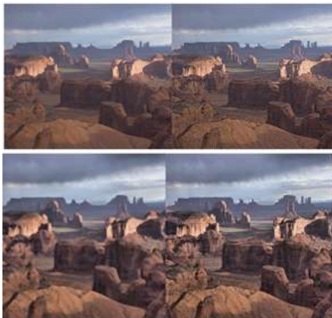
Fig.5.1: Comparison of individual effects of contrast enhancement and detail enhancement. Images from left to right: original, only with detail enhancement, only with contrast enhancement, and with both enhancements.
